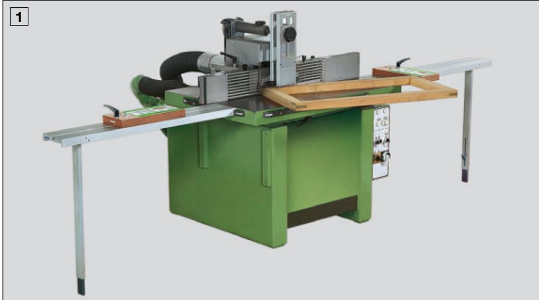
**1** **2** **3** **4** The cross stop prevents kick back when making stopped cuts and allows accurate length stopping.
