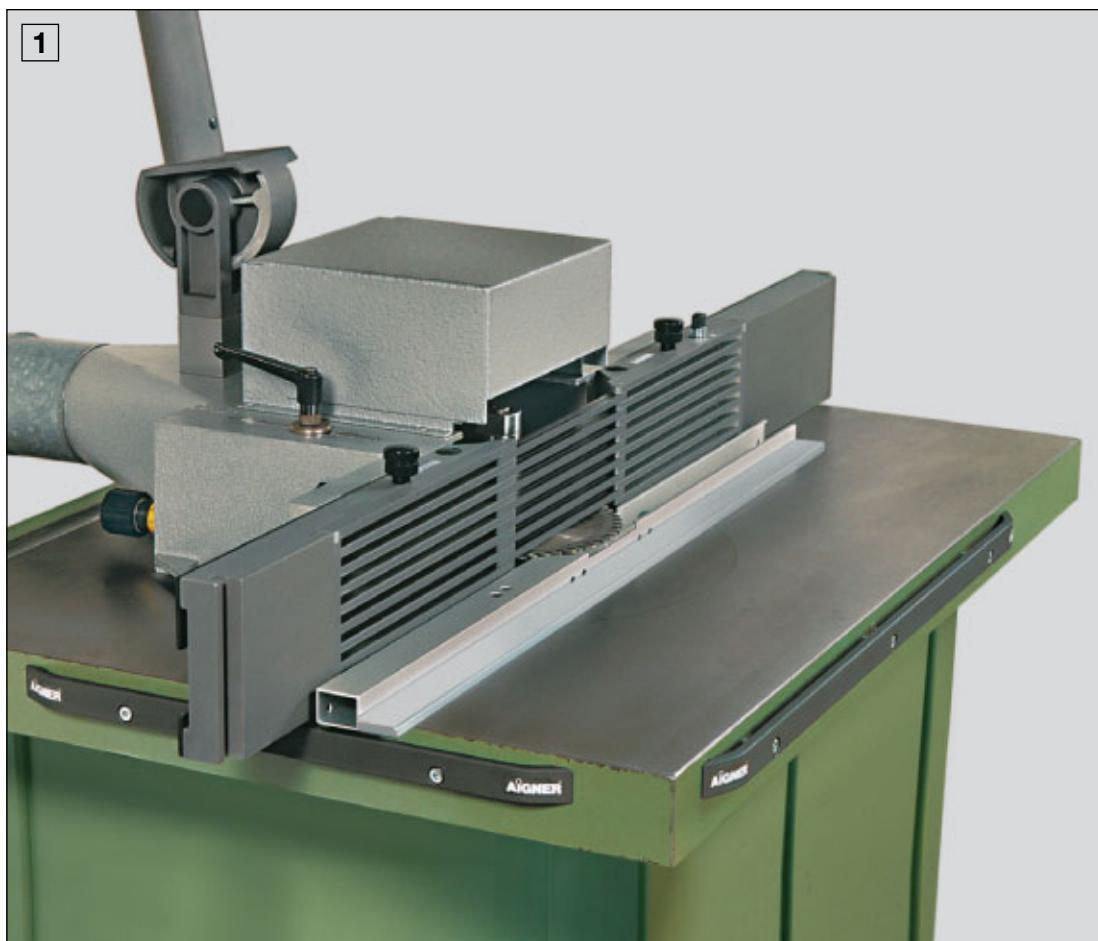
**1** Glassledger attached to the integral fence.
