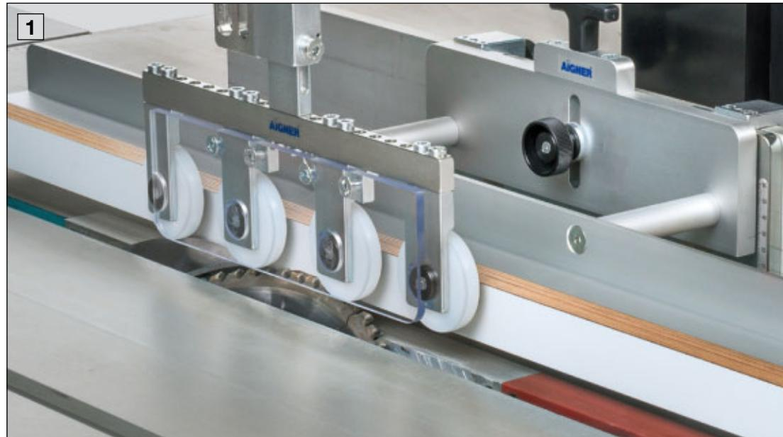
**1** Guiding ledge with protecting wheel. The saw blade is adjusted to the desired bevel cut.
